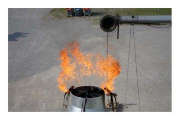
Figure 3: Air-assisted flare tip with sampling collector in TCEQ 2010 test
